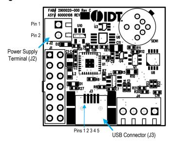
Table 3. Pin Assignments: 2-Post Screw Terminal for Input Power (J2)
