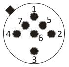
Table 5. Pin Assignments: TO-39 Sensor Socket for SGAS711 (SEN1)
