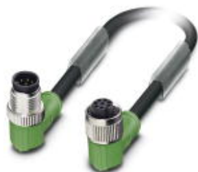
Sensor/actuator cable, 8-position, Variable cable type, Plug angled M12, A-coded, on Socket angled M12, A-coded, cable length: Free input (0.2 ... 40.0 m)
