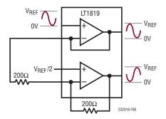
Figure 8. Single-Ended to Differential Driver
