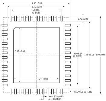
RECOMMENDED SOLDER PAD PITCH AND DIMENSIONS APPLY SOLDER MASK TO AREAS THAT ARE NOT SOLDERED
