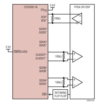
Figure 23. LTC2320-16 Using the LVDS Interface with One Lane
