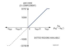
Figure 7. Pseudo-Differential Unipolar Transfer Function
