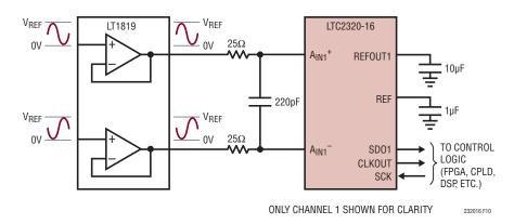
Figure 10. Fully-Differential Application Circuit
