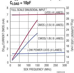
OV<sub>DD</sub> Current vs SCK Frequency,
