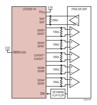
Figure 22. LTC2320-16 Using the LVDS Interface
