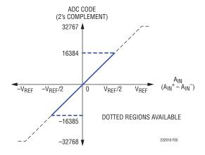
Figure 5. Pseudo-Differential Bipolar Transfer Function
