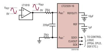
Figure 6. Pseudo-Differential Unipolar Application Circuit
