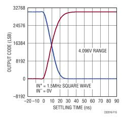
Figure 15. Transient Response of the LTC2320-16
