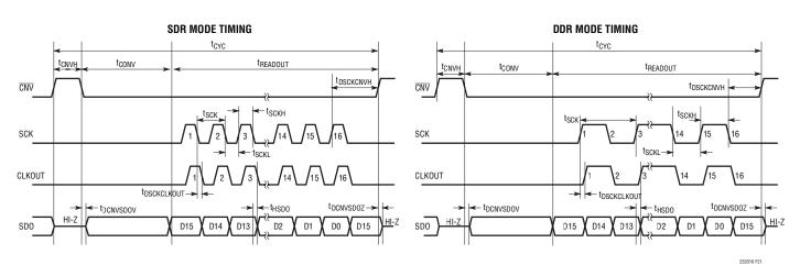
Figure 21. LTC2320-16 Timing Diagram
