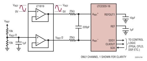
Figure 4. Pseudo-Differential Bipolar Application Circuit
