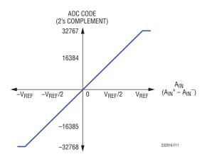
Figure 11. Fully-Differential Transfer Function
